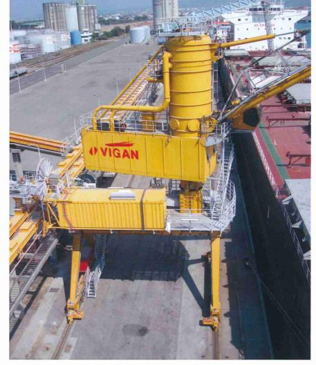
raw materials such as (D)DGS and rapeseed meal. With VIGAN's tailor-made cutting nozzles, many agglomerating raw materials are gently dispersed for onward smooth pneumatic transport.
